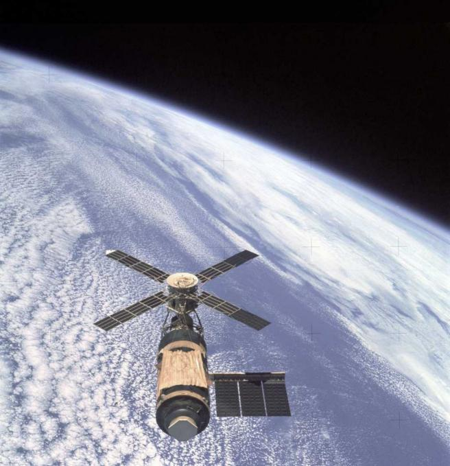
"Skylab" was a 100-ton orbital research and observation platform consisting of an airlock module, docking adaptor, orbital workshop, and a solar and terrestrial telescopic observatory called the "Apollo Telescope Mount".
