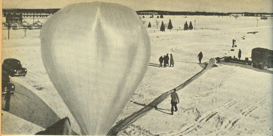
Helium is piped through thin, extruded-plastic tube to form 17-foot bubble. Tapelike line
