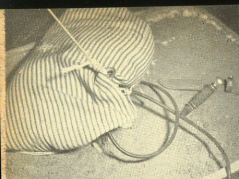
Sandbag at anchor conceals secret device for cutting anchor line electrically at launching. Knife is used in emergency. Balloon will rise above normal airplane traffic in 12 minutes.
