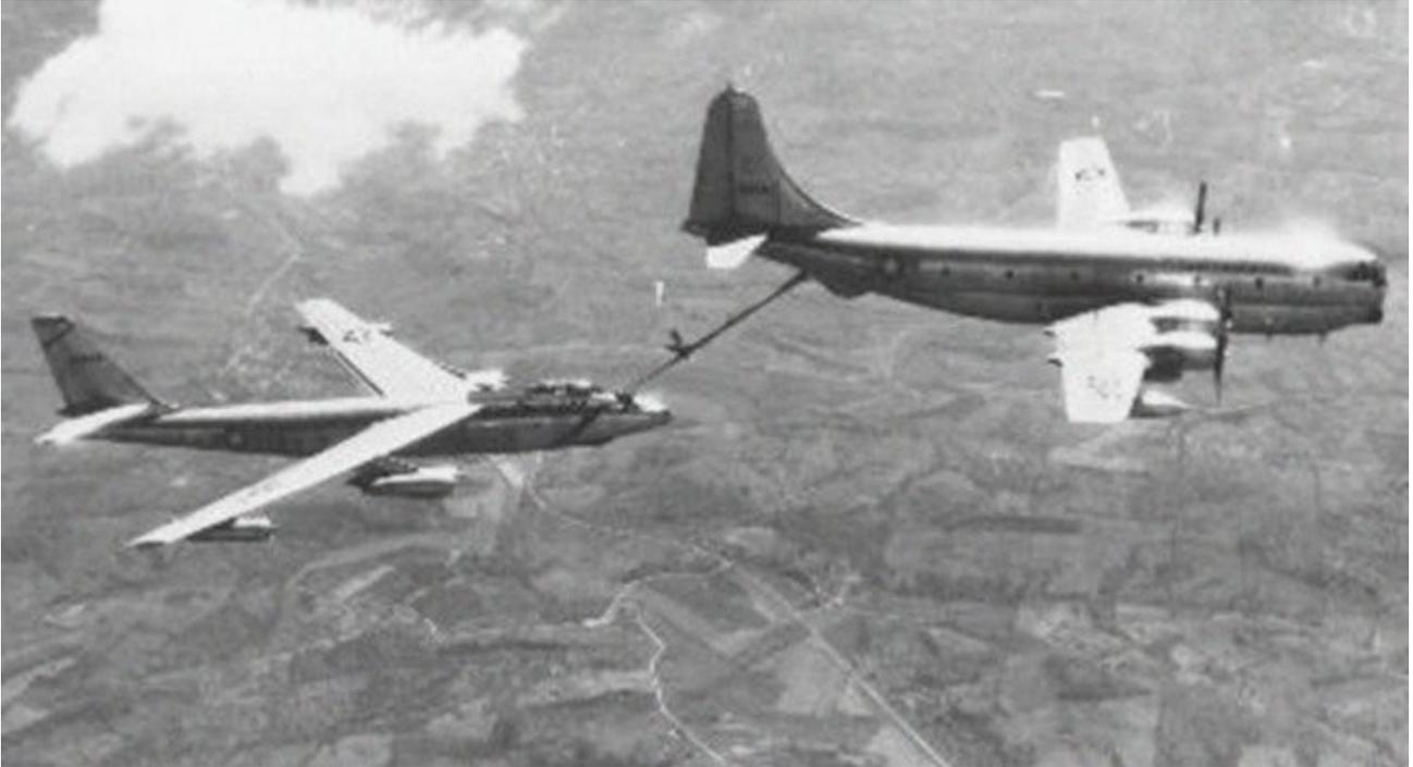
Fig.6 KC-97 Stratotanker refuelling a B-47
