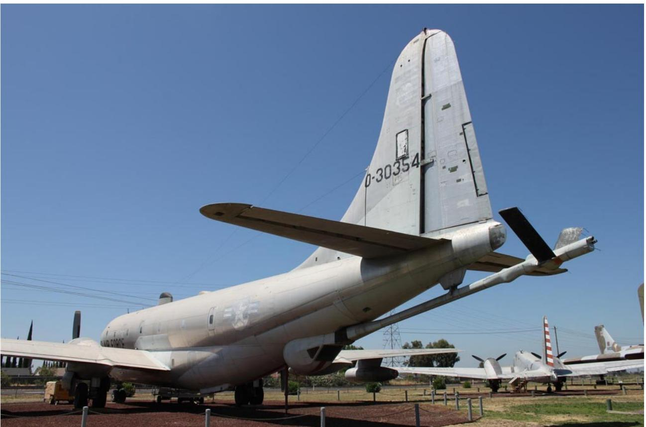
Fig.7 KC-97 showing the boom in stowed position and the boom operator's pod. The receiver light or director light panel is just visible further forward below the wing root
